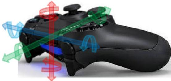
X-axis: the motion on the X-axis (X+/X- direction) is: left → right, right → left;
